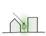
"Fish-bone" roof reduces the feeling of pressure for the surrounding environment and gives a more flexible shape of the building to the visitors.
